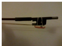
Fig.2 The wireless IMU sensor under the bow frog
